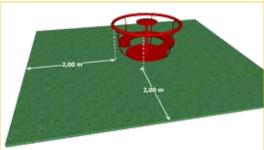
Carousels are playground equipments intended for more than one user at the same time, that can rotate around a central axis without oscillation. The carousels can be of different types:
