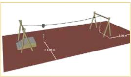
Cableways are equipments whereby the users can travel along a cable under a force of gravity; cableways can be hanging type (equipped with suspension assemblies with a grip for hanging) or seating type.
