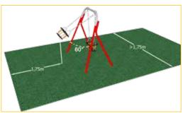
The swing is defined in the standard EN 1176-2 as a moving equipment where the weight of the user is supported below a pivot or universal joint.
